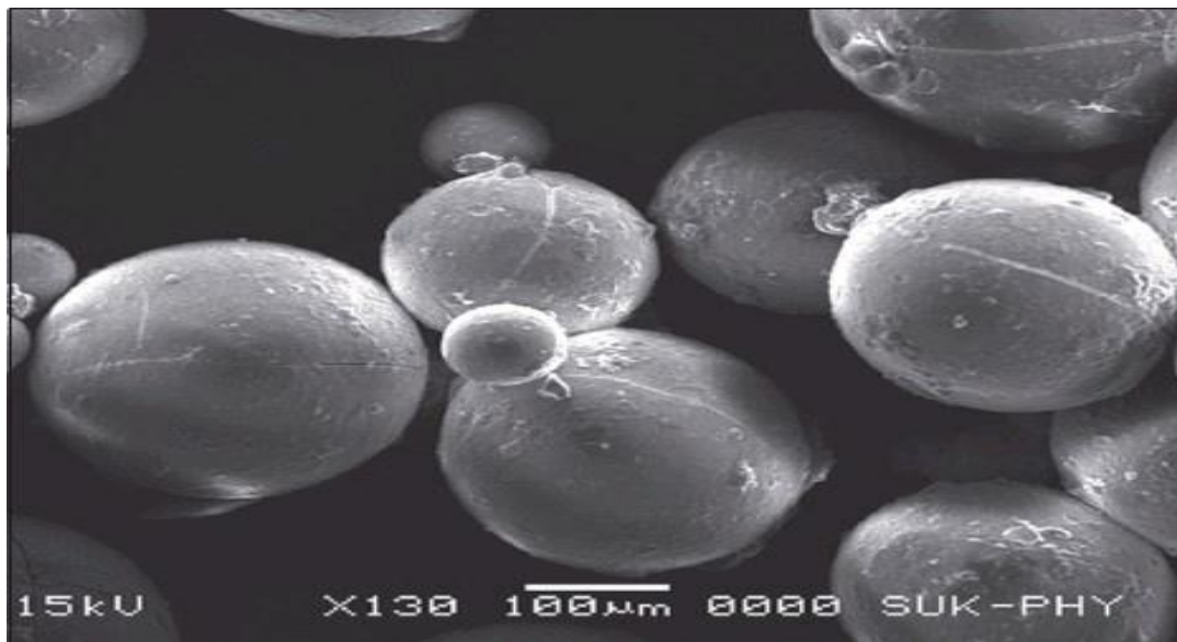
Figure 2: Scanning electron microphotographs of floating microspheres A: the sizerange of microspheres; B and C smoothness of the surface of spherically shaped microspheres.
