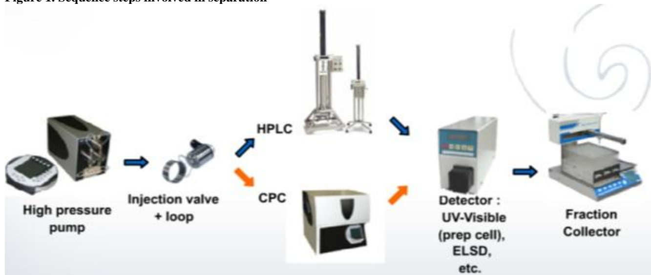
Figure 2. Flow diagram of the two operating modes of the centrifugal chromatograph
