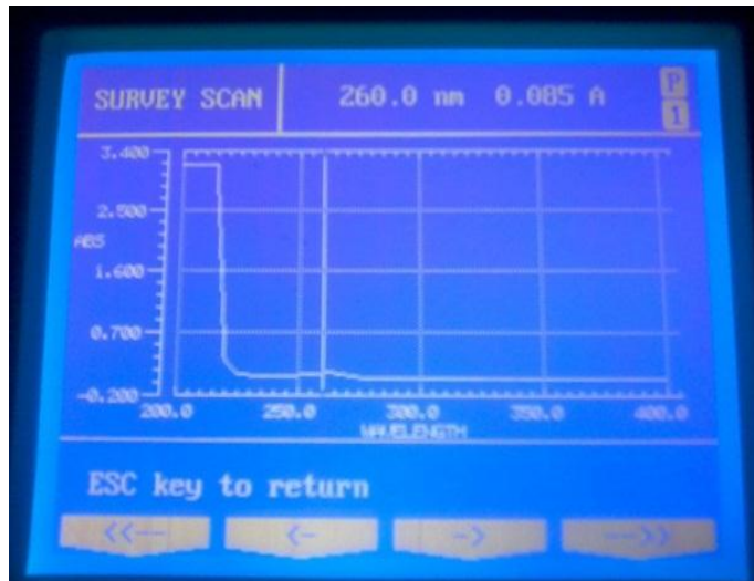
Figure 2. UV Spectrum of Doxylamine showing \lambda_{\max} at 260 nm
