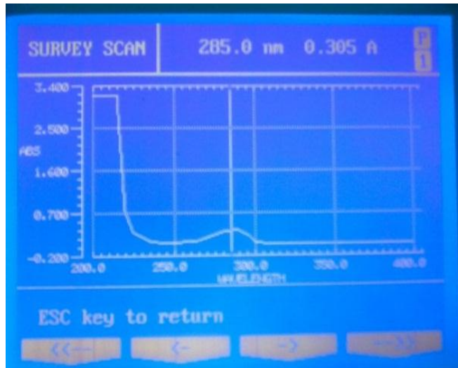
Figure 3. UV Spectrum of Pyridoxine showing \lambda_{\max} at 285 nm
